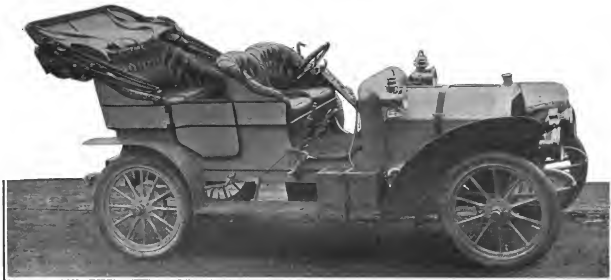
OLDS 1906 MODEL FOUR-CYLINDER MOTOR-IN-FRONT TOURING CAR, BODY FITTED WITH COLLAPSIBLE HOOD.
